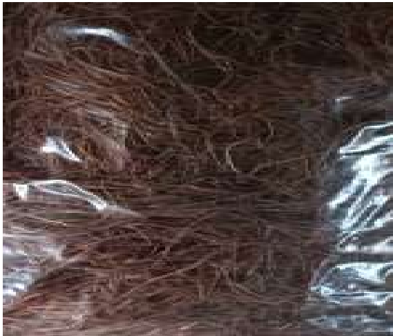
Fig. 1 (b) Extracted dombeya fiber
