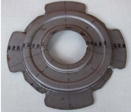
Fig. 8. Metal sheet cover after the first drawing
