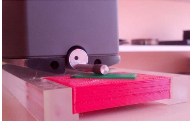
Fig.3 - Specimen holder with a located specimen is correctly positioned within TR 200
