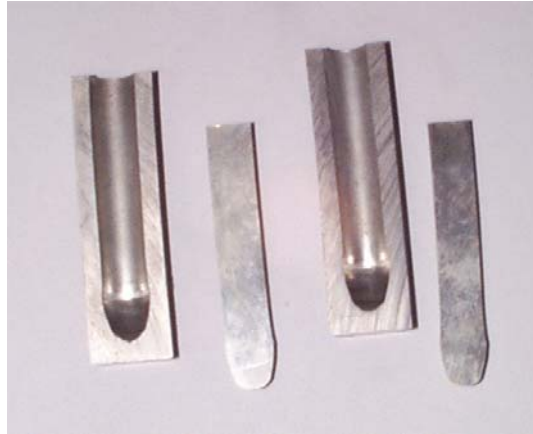
Fig. 6: Extruded specimens (magnesium core and aluminium cage)
