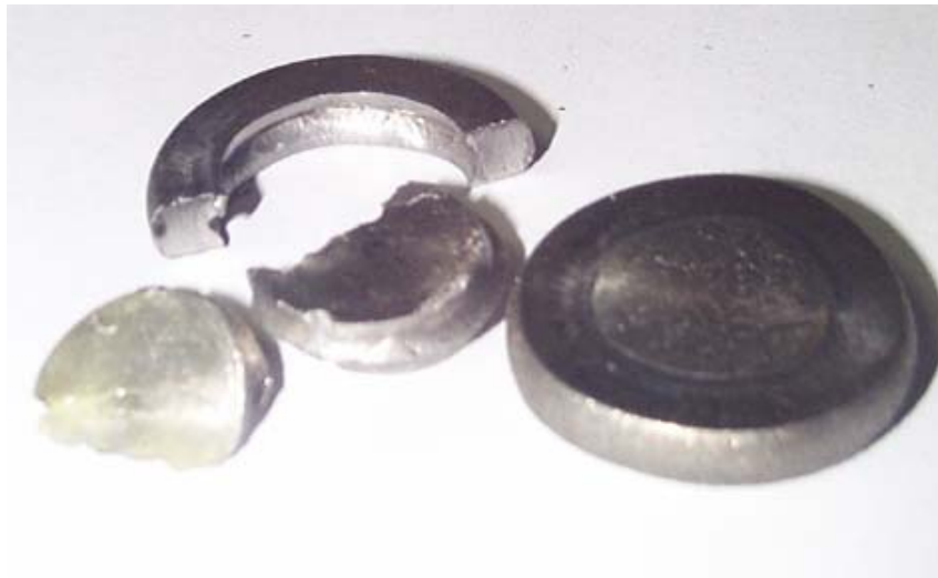
Fig. 3: Cracks in the cylinder when using the steel ring
