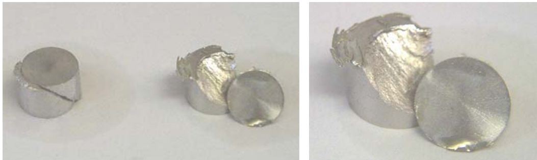
Fig. 1: Upsetting of the magnesium cylinders
