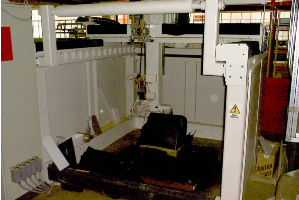
Figure 4. Manufacture the industrial tool for forming plastic part with robot RIKO with control device Stefan PC-106 and control language RRL
