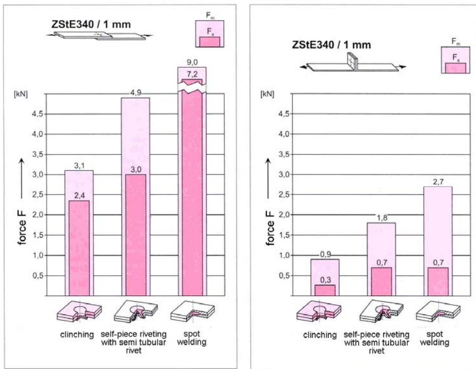
Fig. 15: Test results under quasi static conditions [1]
