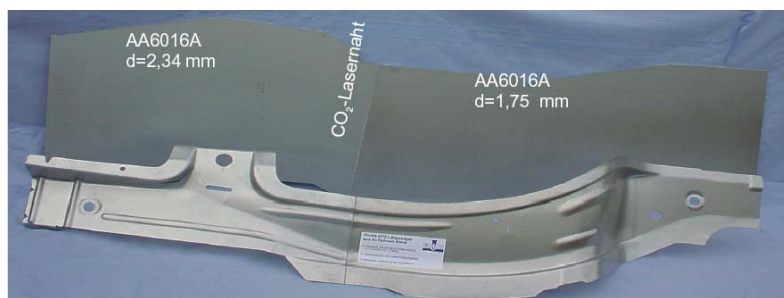
Fig. 5. Part of car body made of aluminum tailored blanks
