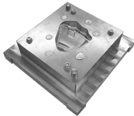
Figure 6: Joining using cast anchors and screws
