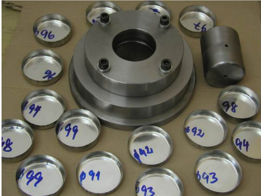
Fig. 1 Test die with shells
