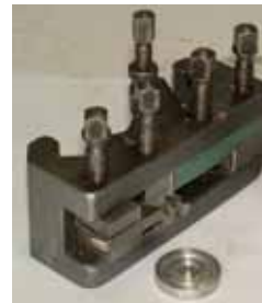
Fig.4.6. Characteristic plate dimensions Fig.4.7. Tool for manufacturing groove plates
