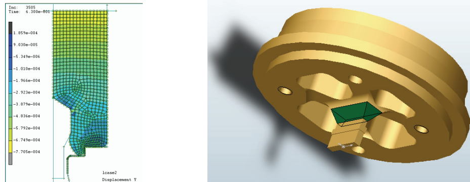
a) FEM model of displacement in y direction b) CAD model of transfer cone on base of FMEA
