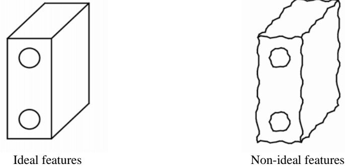
Figure 3 - Ideal model and "Skin-Model" of a Workpiece
