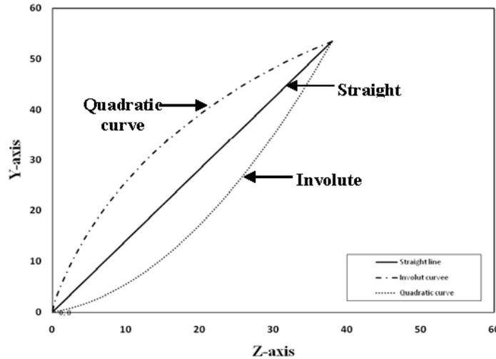
*Fig. 4 - Schematic diagram for the three roller-traces curves used in the first pass*
