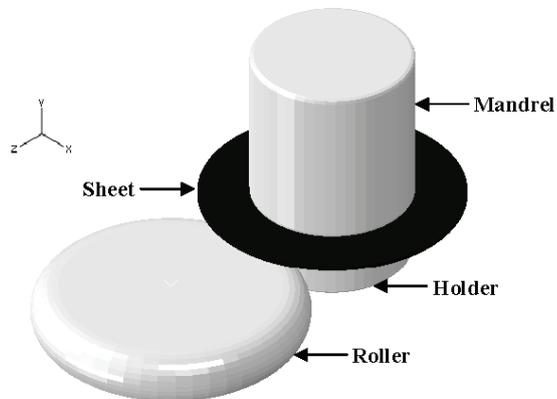
Fig. 2 - 3-D FE model for dual pass conventional spinning
