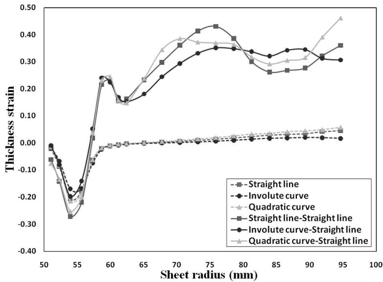
Fig.9. - Thickness strain distributions after first and second pass
