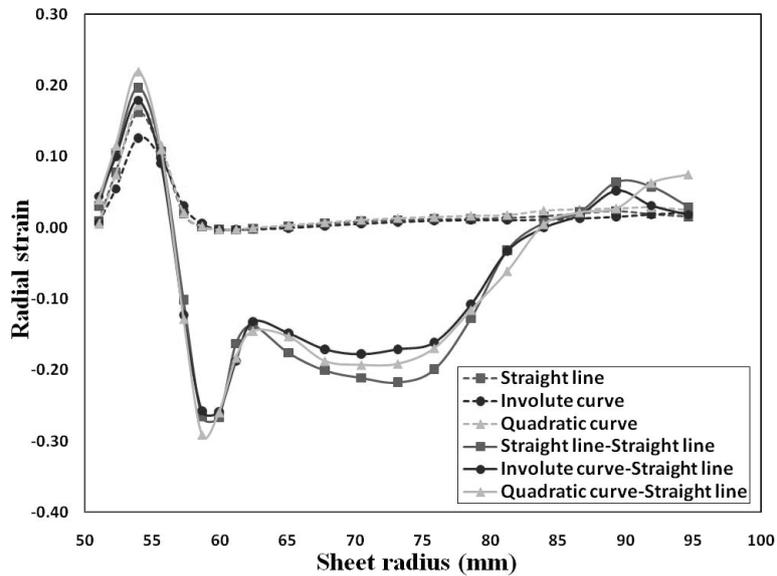
Fig. 7 - Radial strain distributions after first and second pass
