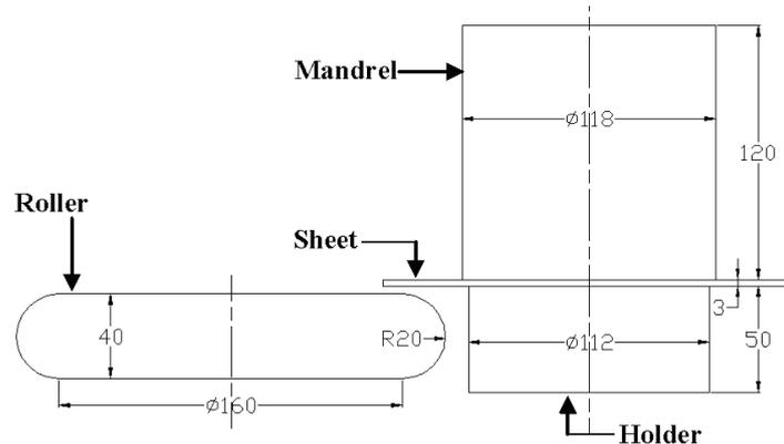
Fig. 1 - Geometries and dimensions of the model (all dimensions in mm)
