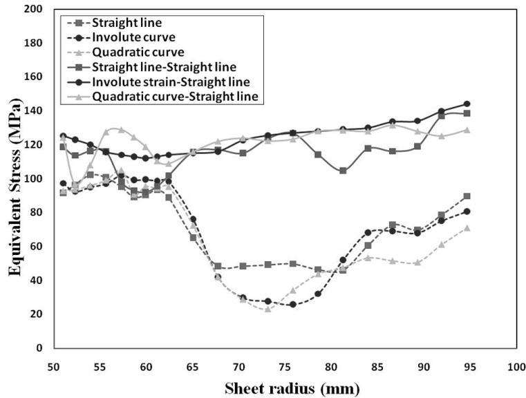
Fig. 6 - Equivalent stress distributions after first and second pass
