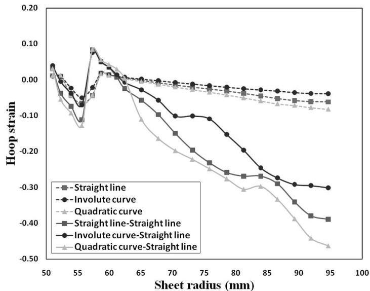
Fig. 8 - Hoop strain distributions after first and second pass
