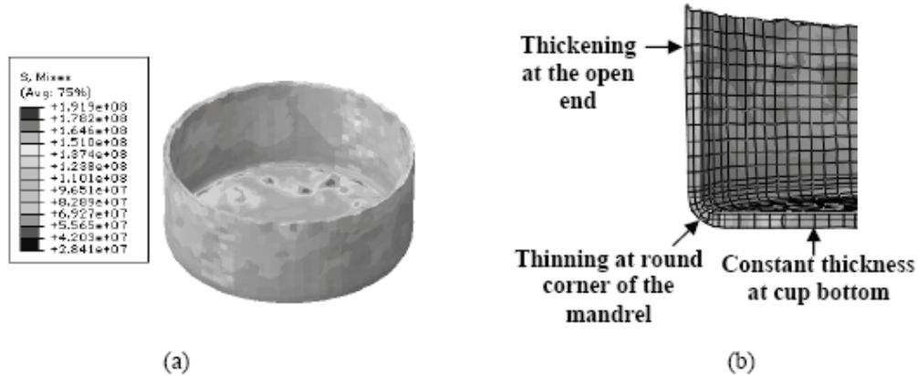
Fig. 3 -. (a) Von Mises stress in the fully deformed cup, and (b) a section through the cup with the FE mesh superimposed revealing the local thinning.
