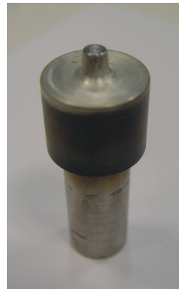
Fig. 5 - Tool made of steel č.4751
