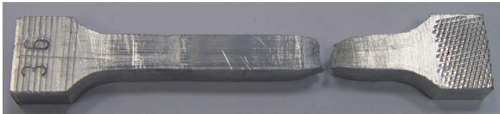
Fig. 13 - A stretched test piece, cut from the y - direction
