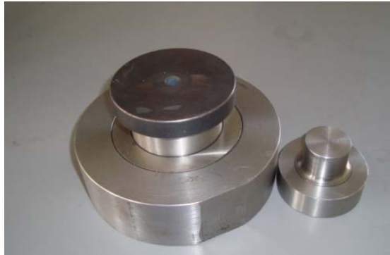
Fig. 3 - Compressing tool for die
