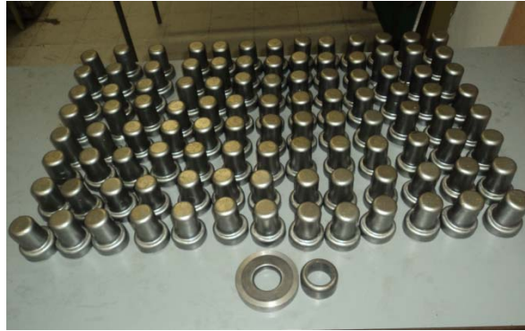
Fig. 5 - The die, the blank holder and deep drawn pieces
