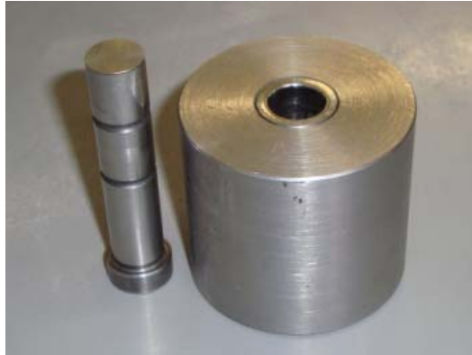
Fig.1 - Tool for compacting of test pieces
