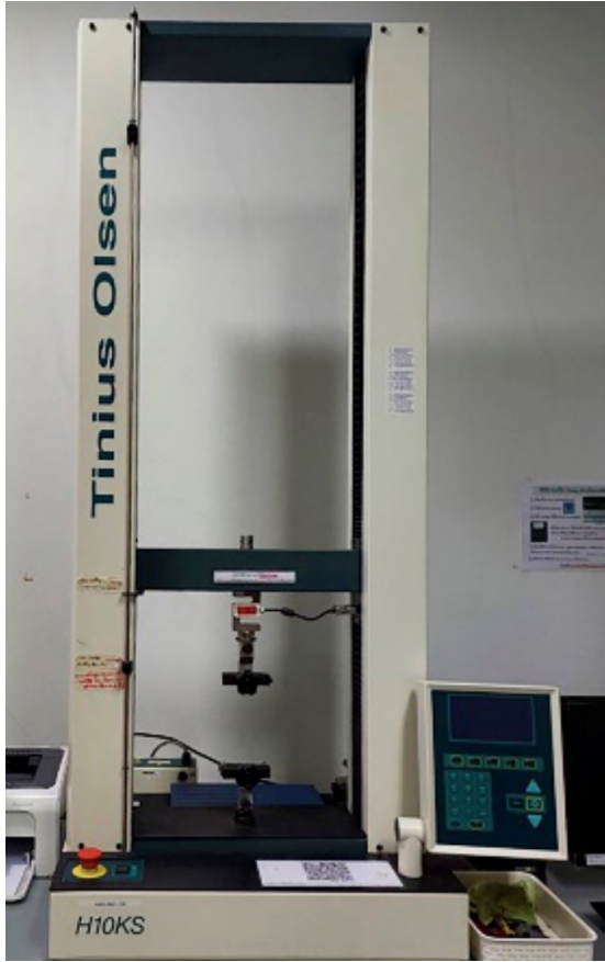
» Figure 4: Compression test with Universal testing machine
