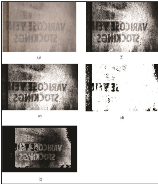
» Figure 5: (a) Original image (b) RGB to Gray Converted image (c) Histogram Equalized Image (d) Foreground Image (e) Detected Showthrough Pixels
