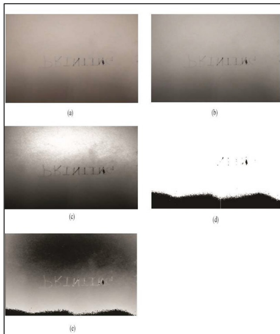
» Figure 8: (a) Original image (b) RGB to Gray Converted image (c) Histogram Equalized Image (d) Foreground Image (e) Detected Strikethrough Pixels
