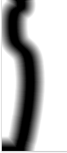
» Figure 7: Illustration of an example of the distance map that is stored in the blue channel of the shape map.
