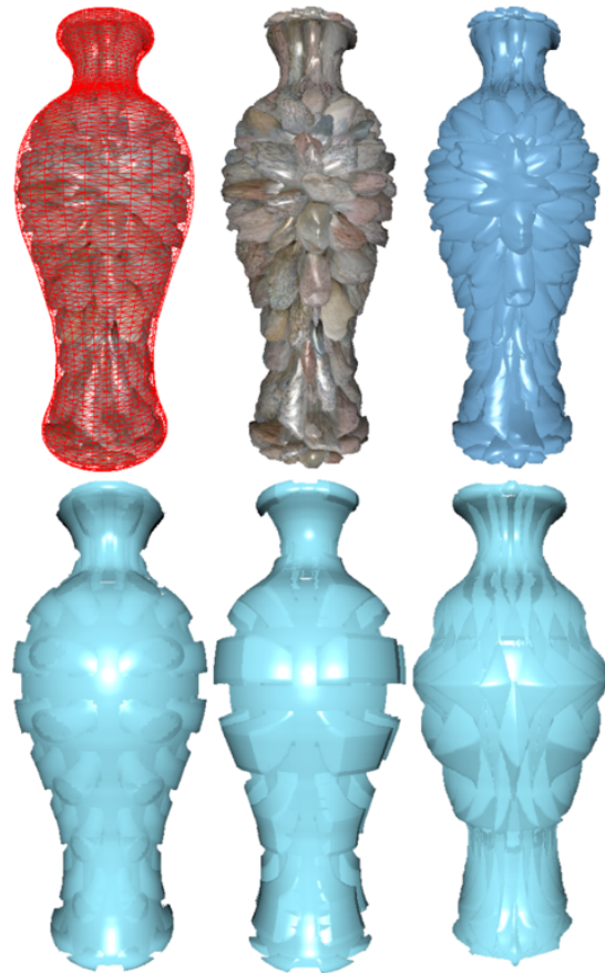
» Figure 41: Rendering of a vase with the cone tracing technique with correct silhouette by highlighting the basic polygonal mesh and by using different depth maps and different depth values
