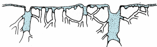
» Figure 3: Capillary structure of paper and absorption of ink
