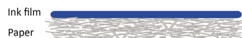
» Figure 1: Newly printed ink film on the top surface of the paper
