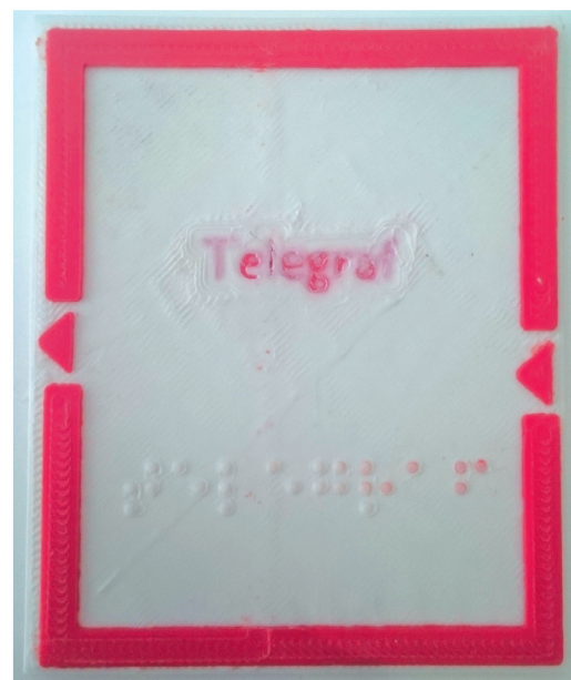
» Figure 5: Complex mesh of the 3D model of text and (a) unsuccessful attempt of simultaneous 3D printing of Braille and Latin letters (b)
