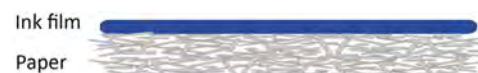
» Figure 1: Newly printed ink film on the top surface of the paper
