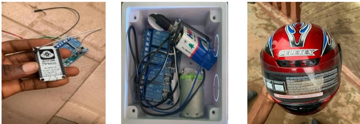
Fig. 11 (a) NodeMCU connection to both relays; (b) Prototype smart helmet connections; (c) Back view of the rider and DC motor.
